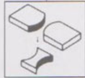
平钢双边圆弧剪切 The arcshears the flat steel doubling piece
